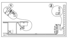
The waste connection must be at a height of between 30 cm (minimum) and 100 cm (maximum) from the bottom of the dishwasher.
